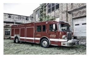
Rescue #6 – 2013 Spencer/Spartan Rescue with 750 gallons of water. This is the first out machine on all accidents and second out of all residential fires. This machine also provides mutual aid to area departments for accidents.
